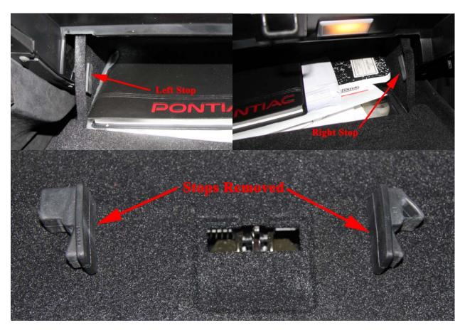
The first step is to gain access to the area behind the glove box to see if your car has a potential problem. This is very straightforward if you know how to do it. The first step is to open the glove box past the rubber stops. There is one rubber stop on each side of the glove box. I like to just work the rubber stops out of the door. To do this, grasp them from the inside of the glove box and pull them towards the inside of the globe box and down. They will slide out pretty easily.
