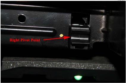
hand side. This will cause the right pivot point to snap out of the clip. It does not take much force to pull this loose, so don't overdo it. Once the right pivot point is free, simply slide the glove box to the right to free it from the left pivot point. At this point the glove box will be totally free and can be set aside.
